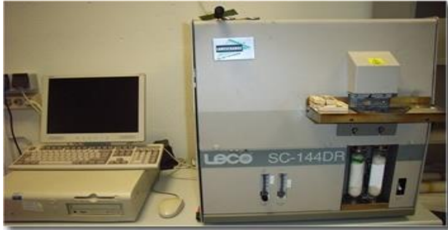
Figure: 1 LECO SC-144DR Sulphur-Carbon Analyzer
